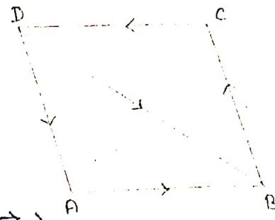
The forces in the first brackets are in equilibrium by the polygon of forces (here the square ABCD) and the forces in the second brackets are in equilibrium by the triangle of forces (here the triangle BCD). (5)
